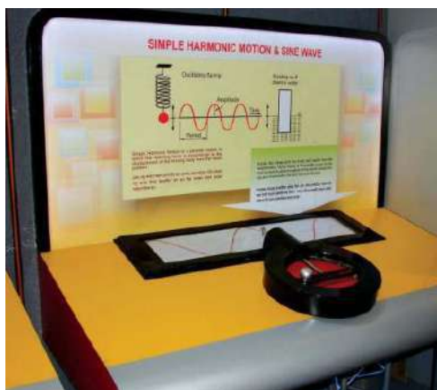
Figure 38: An interactive exhibit to convert circular motion into a Simple Harmonic Motion and trace a Sine Wave.
