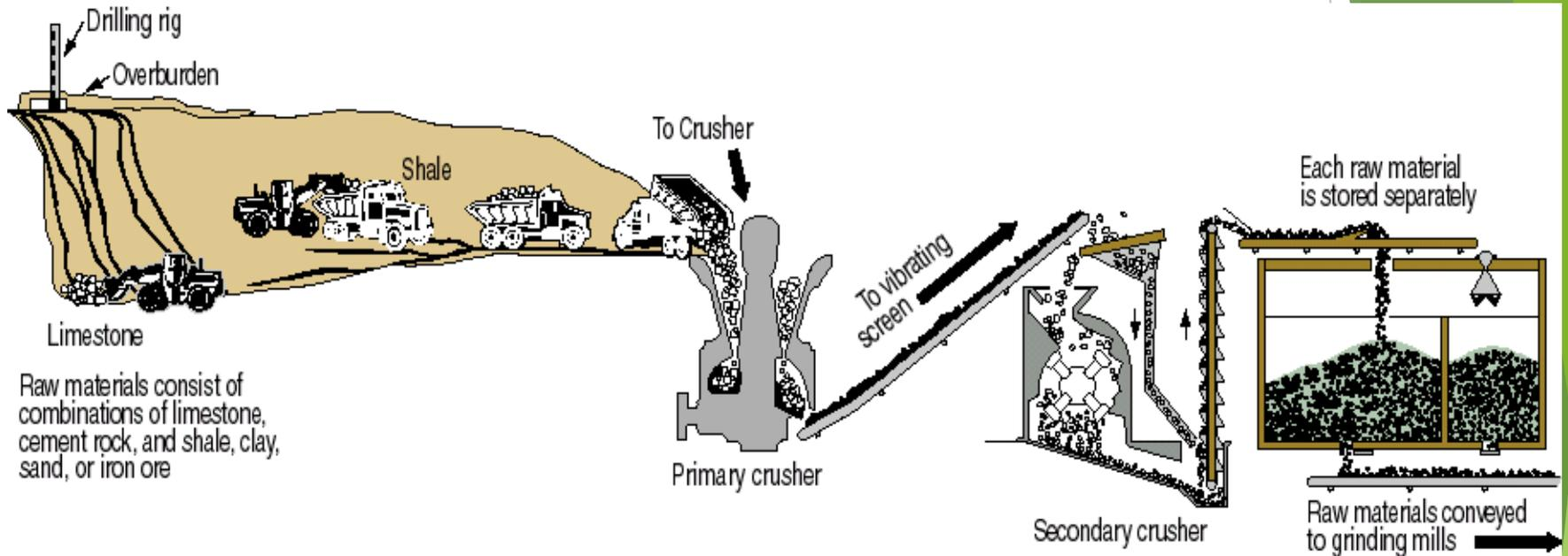
**1. Stone is first reduced to 125 mm (5 in.) size, then to 20 mm (3/4 in.), and stored.**
