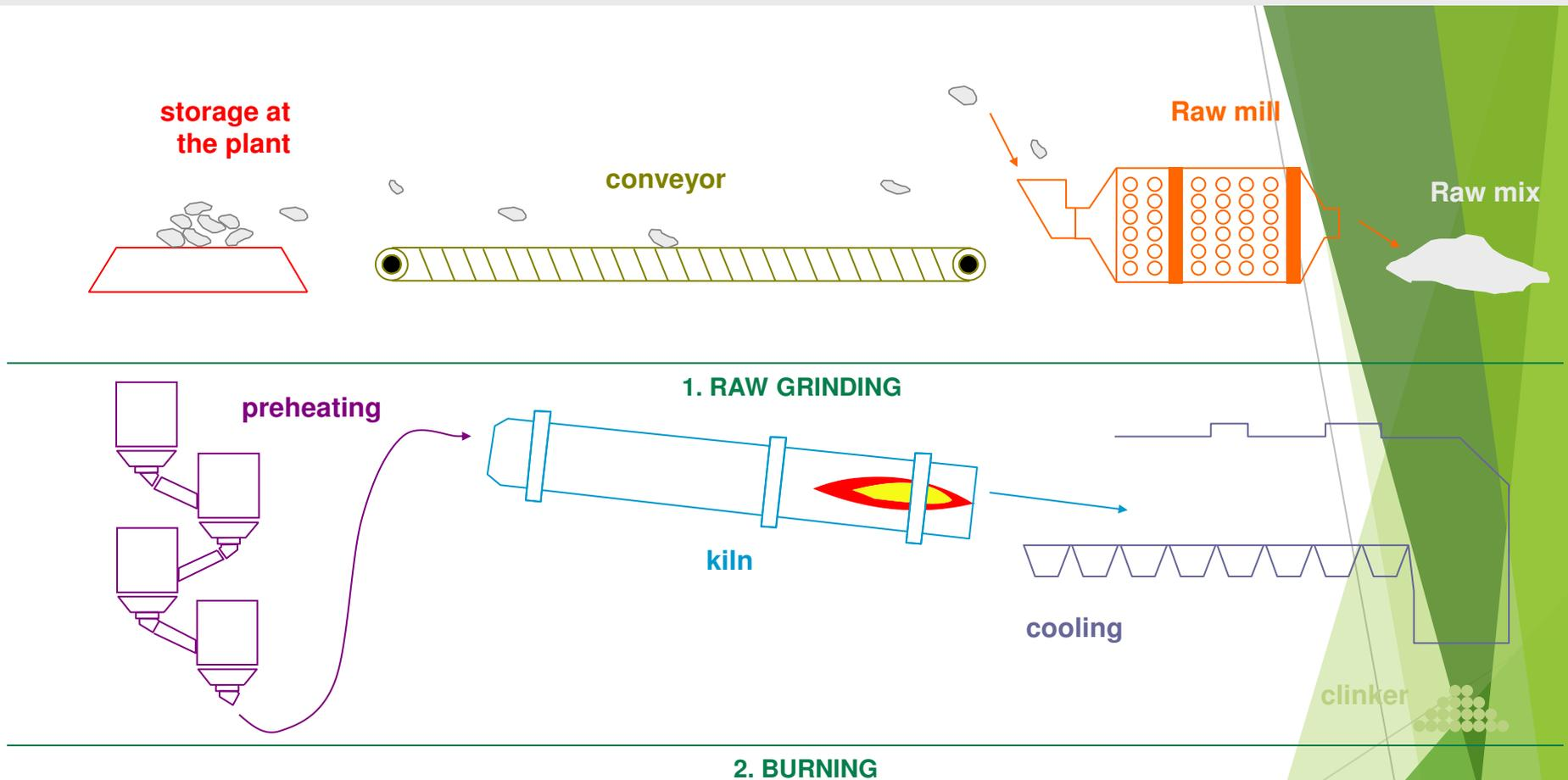
**1. RAW GRINDING :** The raw materials are very finely ground in order to produce the **raw mix**.
